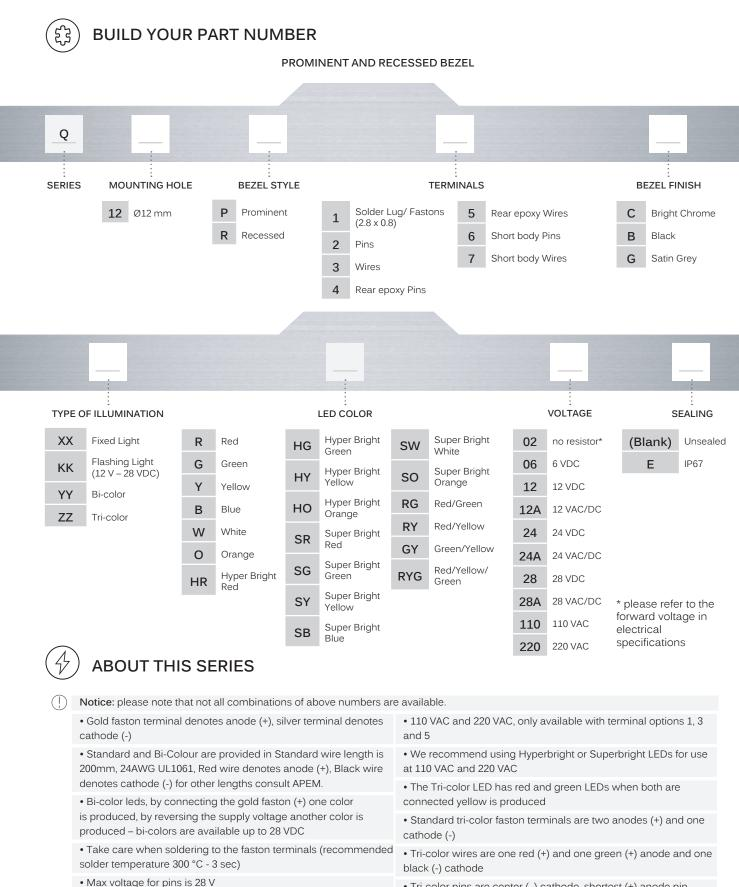
• Tri-color are not available with terminal option 1 and behind panel epoxy sealed with pins to option 4 and wires to option 5.
